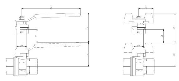
Dimensions Y, y, Y1 and y1 are additional to dimension H on the relevant valve drawing
