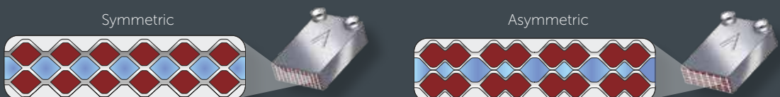
Cross-section of the channels inside of a symmetric and asymmetric plate heat exchanger
